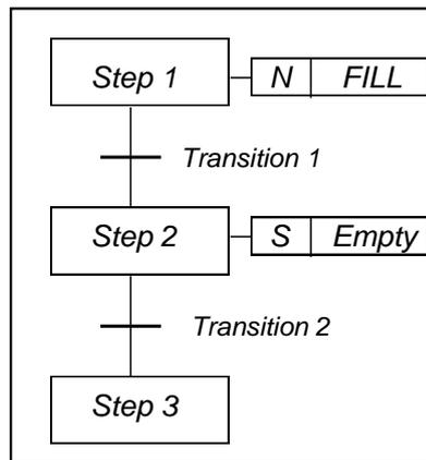
SFC describes graphically the sequential behavior of a control program. With this it structures the internal organization of a program, and helps to decompose a control problem into manageable parts, while maintaining the overview.
