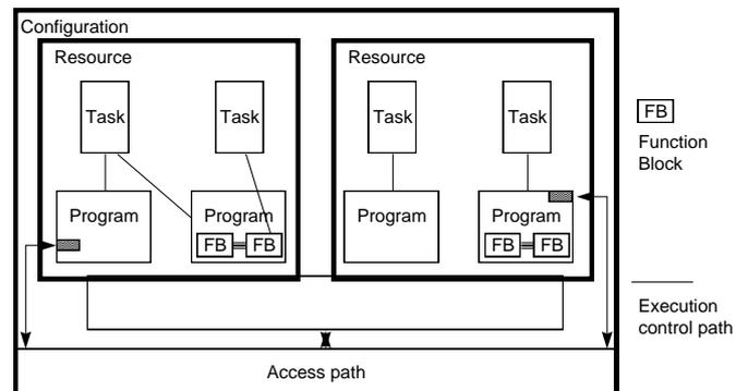
At the highest level, the entire system required to solve a particular control problem can be formulated as a *Configuration*, including the arrangement of the hardware, memory addresses for I/O channels and system capabilities.
