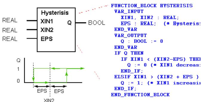
The Function Block above (on the left side) is represented here in the programming language Function Block Diagram. The Function Block has the name Hysteresis. It has three inputs on the left, named XIN1, XIN2 and EPS, all of datatype REAL. It has one output, on the right, called Q, of type BOOL.
