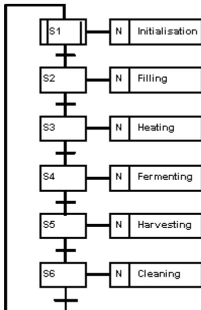
We start at the top with the Initialization: since we do not know the status of the system when we first switch it on, we must check the position of the valves, etc. Then we start filling till the right level has been reached.
