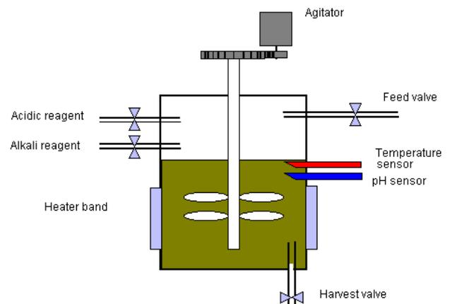
All external interfaces are defined here (step 1). There is a large vessel, which can be filled (Feed Valve) with the liquid, can be heated with the heater band (cooling via convection), can be stirred via the motor, and where acid and alkali fluid can be added into the vessel.
