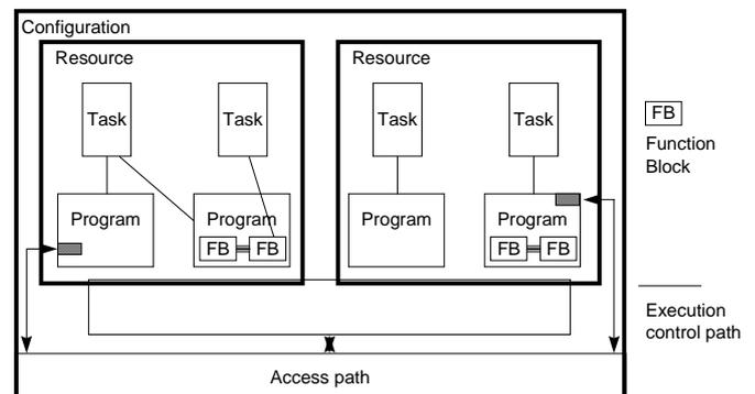
At the highest level, the entire software required to solve a particular control problem can be formulated as a *Configuration*. A configuration is specific to a particular type of control system, including the arrangement of the hardware, i.e. processing resources, memory addresses for I/O channels and system capabilities.
