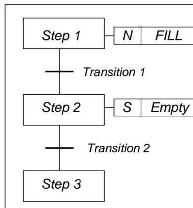
SFC describes graphically the sequential behavior of a control program. It is derived from Petri Nets and IEC 848 Grafset, with the changes necessary to convert the representation from a documentation standard to a set of execution control elements.
